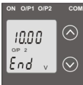
This screen allows the user to set the End value of Output 2, (considered as DC Voltage) for dual output. The End value of Voltage Output fixed at 10V.
