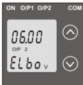
Pressing the " √ Down" key will enter the "New / Change Elbow value of the Output 2 edit" mode. Pressing " ^ Up" key will confirm the present value as Elbow value of the Output 2 and exit setup menu.
