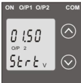
Change Start value of the Output 2”. Pressing the “ ^ Up” key will confirm New Start value of the Output 2 and advance to the Elbow value of Output 2 setting (section 3.1.5.2.3) or exit setup menu, If elbow not enabled.
