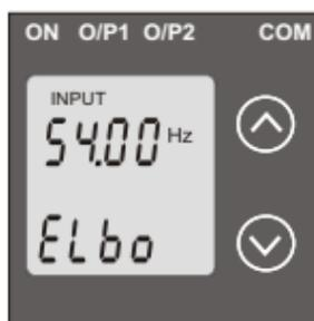
This screen appears only when the Elbow function is enabled & allows the user to set the Elbow value of the Input. Allowable range of Elbow value of input is between (start value + 0.015\* End value) to 0.985\* end value
