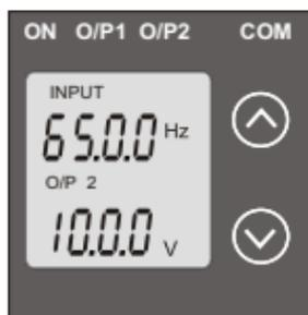
Screen 6 : Frequency Input and Output 2 as Current
