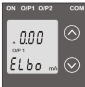
Pressing the “ √ Down” key will scroll the value of the first digit from 0 through to 1, the value will wrap from 1 round to 0 depending on the set End value of Output. Pressing the “ ^ Up” key will advance the operation to the next digit and set the first digit, in this case to “1”.
