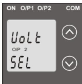
This screen allows the user to set the output 2 type as Voltage or Current for dual output transducers
