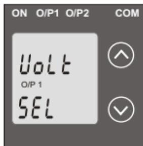
Pressing " √ Down" key will re-enter into Output 1 Type Edit mode.
