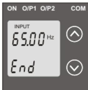
Pressing the “ v Down” key will enter the “New/Change End value of Input edit” mode. Pressing “ ^ Up” key will confirm the present value as End value of Input and advance to the Start value of Input setting (section 3.1.4.2).
