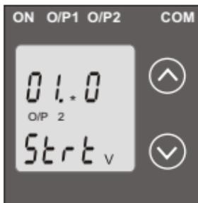
third digit from 0 through to 9, the value will wrap from 9 round to 0. Pressing the “ ^ Up” key will advance the operation to the next digit and set the third digit, in this case to “5”.
