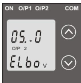
Enter New / Change Elbow value of the Output 2, second digit entered, \ prompting for third digit. (\*Denotes that digit will be flashing).
