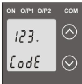
Enter Password, third digit entered, prompt for fourth digit. (\*Denotes that digit will be flashing). Pressing the " √ Down" key will scroll the value of the fourth digit from 0 through to 9, the value will wrap from 9 round to 0.
