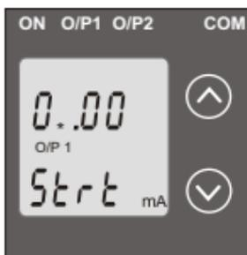
Enter New / Change Start value of the Output 1, first digit entered, prompting for second digit. (\*Denotes that digit will be flashing). Pressing the "v Down" key will scroll the value of the second digit from 0 through to 4, the value will wrap from
