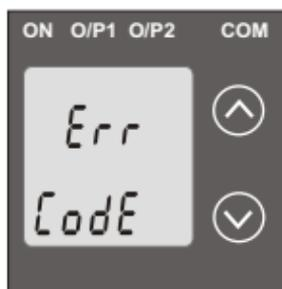
This screen is displayed ,when the unit has not accepted the Password entered.
