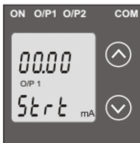
Pressing the “ v Down” key will re- enter to the “New / Change Start value of the Output 1”.
