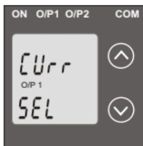
This screen allows the user to set the output 1 type as Voltage or Current.
