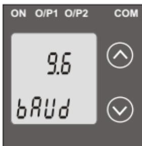
Pressing " √ Down" key will be re-enter into the. "Baud Rate Edit" mode
