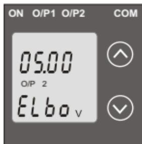
Pressing the " v Down" key will re-enter to the "New / ChangeElbow value of the Output 2".
