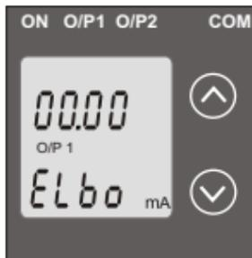
Pressing the “ √ Down” key will enter the “ New/Change Elbow value of the Output 1 edit” mode. Pressing “ ^ Up” key will set the present value as Elbow value of the Output 1 and advance to the Output 2 characteristics setting(section 3.1.5.2).
