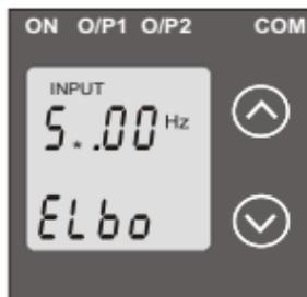
Pressing the “ v Down” key will scroll the value of the second digit from 0 through to 9, the value will wrap from 9 round to 0 depending on the set End value of Input.
