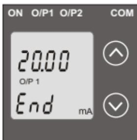
This screen allows the user to set the End value of Output 1, (considered as DC Current). The End value of Current Output fixed at 20mA.
