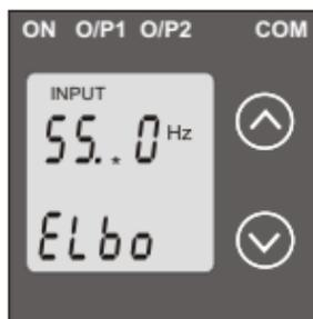
Pressing the “ √ Down” key will scroll the value of the third digit from 0 through to 9, the value will wrap from 9 round to 0 depending on the set End value of Input. Pressing the “ ^ Up” key will advance the operation to the next digit and set the third digit, in this case to “0”.
