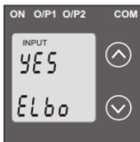
Pressing "∨ Down" key will re-enter into Elbow function of Input Edit mode.
