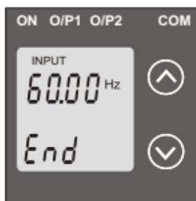
Pressing the "∨ Down" key will re- enter to the "New / Change End value of Input".
