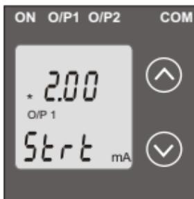
(\*Denotes that digit will be flashing). Pressing the "v Down" key will not affect the first digit. It always remains 0. Pressing the " ^ Up" key will advance the operation to the next digit and set the first digit, in this case to "0".
