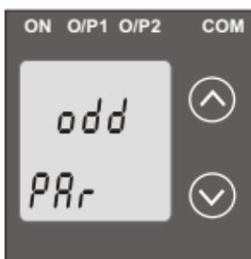
This screen allows the user to set Parity & number of stop bits of RS 485 port.
