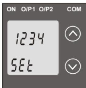
Pressing " √ Down" key will enter to the "New / change Password" entry stage (section 3.1.1.2). Pressing the " ^ Up" key will advance to the Communication parameter selection (section 3.1.2).
