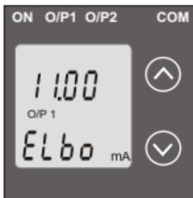
Pressing the " √ Down" key will re-enter to the "New / Change Elbow value of the Output 1".
