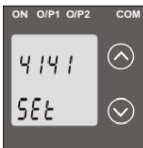
Pressing the “ v Down” key will re- enter to the “New Password” entry stage. Pressing the “ ^ Up” key will confirm New Password and advance to the Communication parameter setting (Section 3.1.2).
