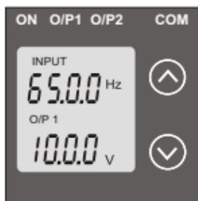
Screen 4 : Frequency Input and Output 1 as Current
