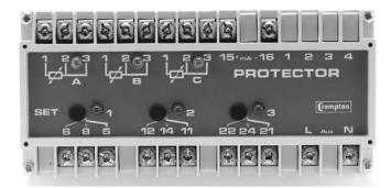
The Crompton Hot Spot 3 relay accepts up to three inputs from resistance temperature detectors (RTD) and provides up to three user adjustable trip points which can be used to initiate alarms, cooling systems or shutdown.
